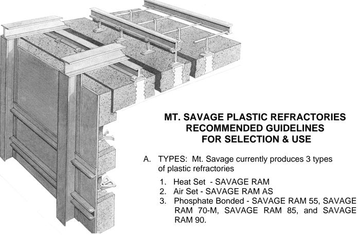
Heat setting plastics require firing to develop a ceramic bond. Air setting plastics contain an organic binder that will harden on air-drying but also develop a ceramic bond at higher temperatures.
