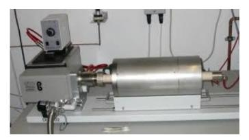
A dilatometer that measures the length of a refractory sample as it is heated through a temperature range.
