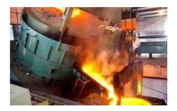
An electric arc furnace (EAF) teeming into a steel ladle. Production of both EAF steel and integrated steel is down country wide.
