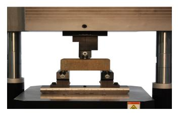
Modulus of Rupture being tested on a refractory sample.
