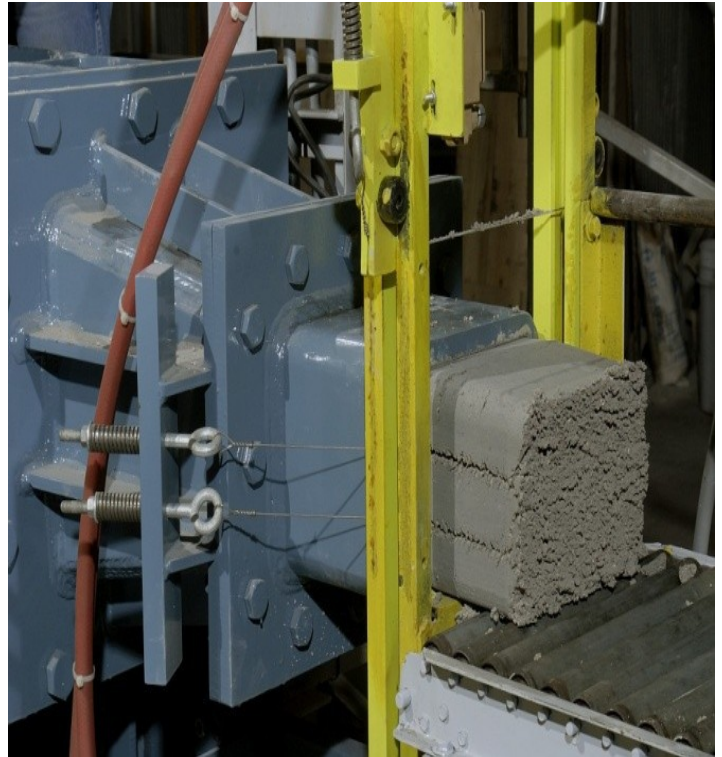
Clots of plastic being extruded from the improved plastic line at Curwensville, PA.
